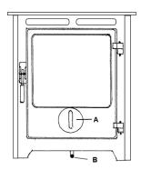
Primary air control (A) on front of door. Secondary air control (B) below the ash shelf
